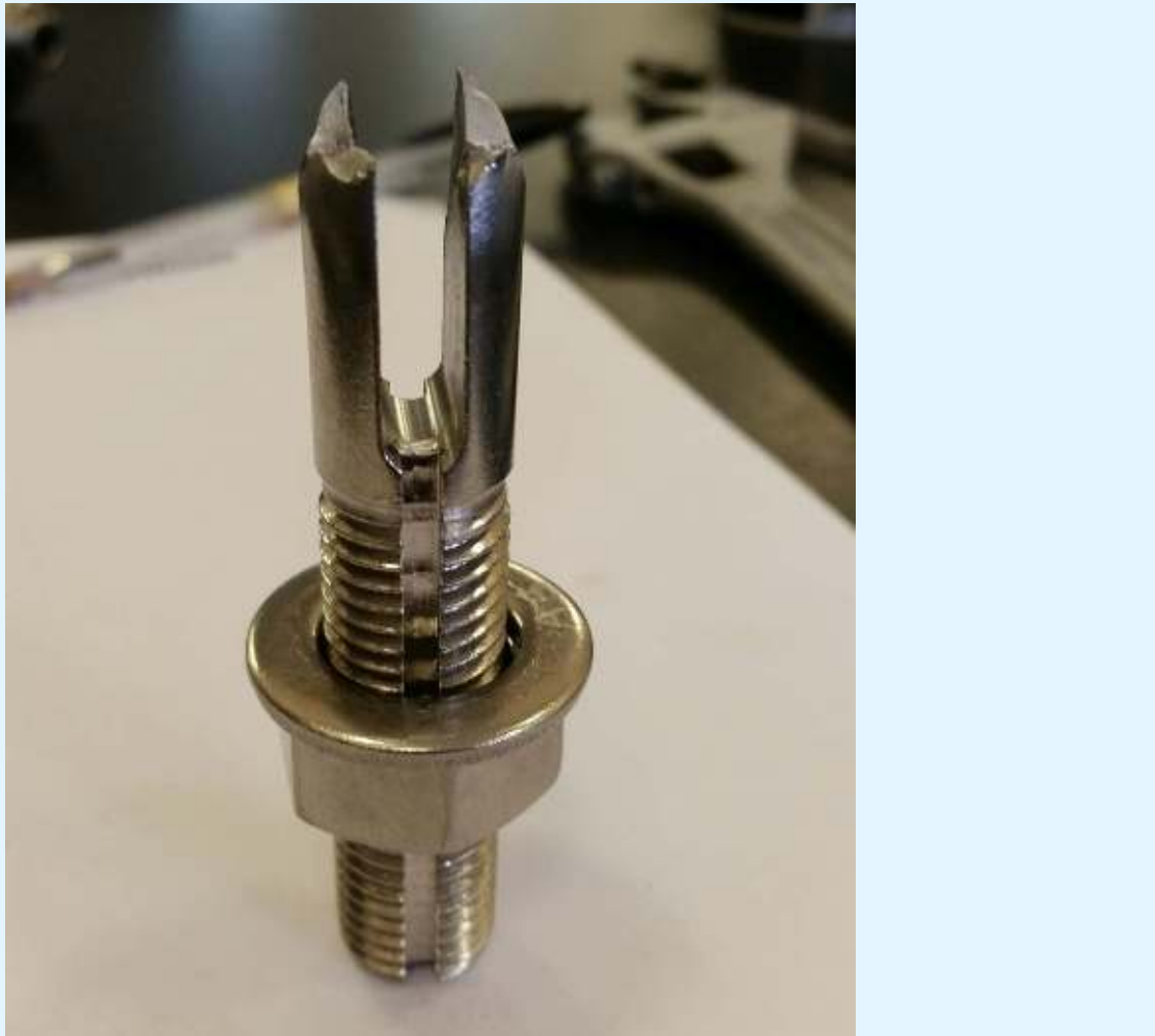
Figure 3.2 Completed tension test
