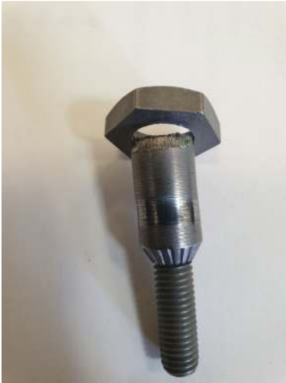
Figure 3.4 Tension test M8, carbon steel
