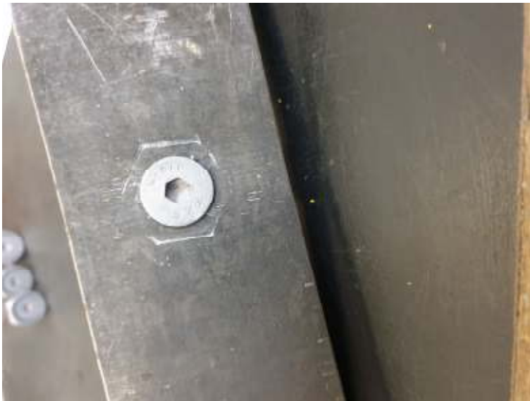
Figure 3.3 Tension test plate, M8, carbon steel
