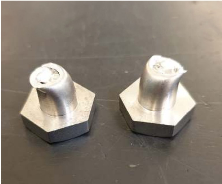
Figure 2.1 Shear test M6, stainless steel
