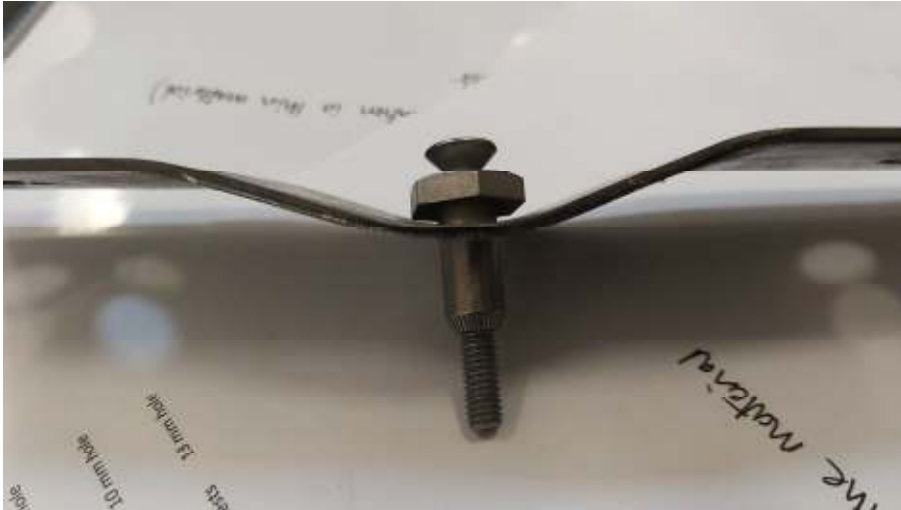
Figure 5.1 Typical pull-through test
