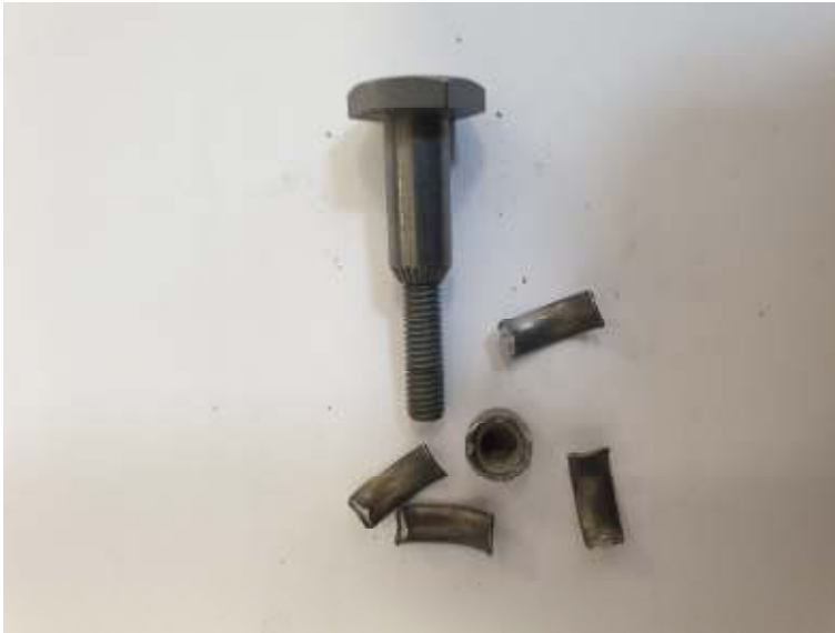
Figure 3.2 Tension test M5, carbon steel
