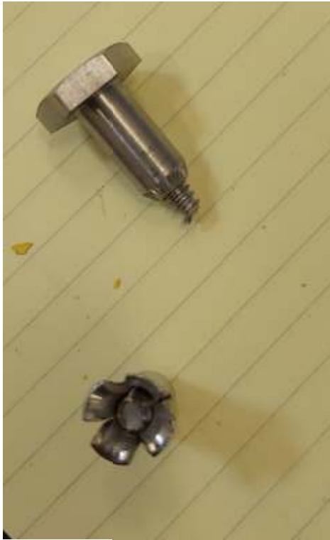
Figure 3.1 Tension test M6, stainless steel
