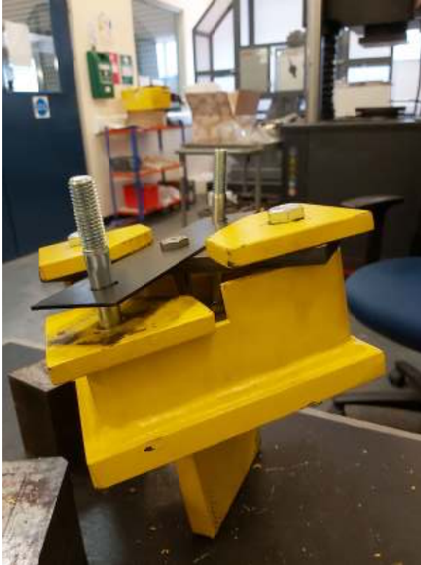
Figure 1.4 Disassembled test rig (pull-through test)
